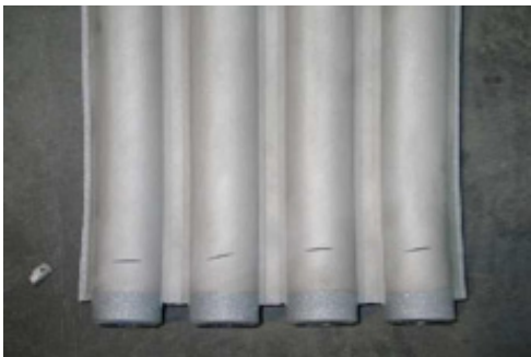
Figure 3: Colmonoy coated Super heater element for a WtE plant in the UK, coated boiler wall panel [2]
