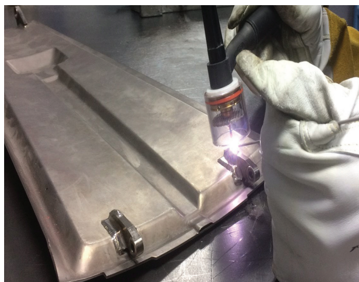
Aerobrazed Engineer using InterPulse GTCAW on a Titanium Divergent Petal
